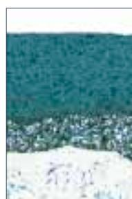
Cross section of Flygt epoxy coating
